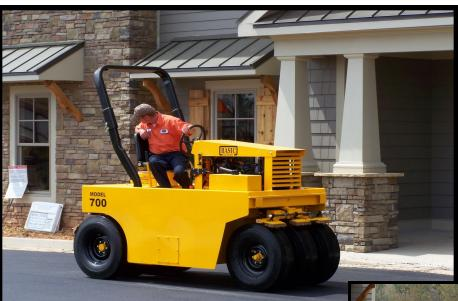
Overall Dimensions: Length: 112" Width: 51" Height: 74" Wheel Base: 82" Chassis Clearance: 9"
